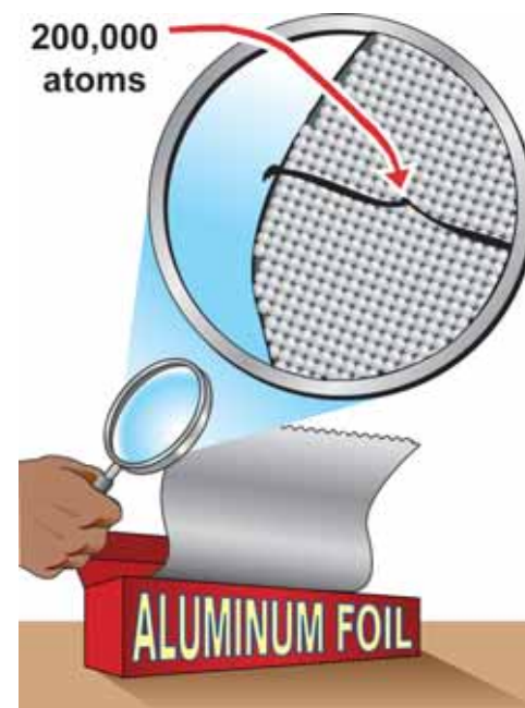
Figure 3.3: Even a thin sheet of aluminum foil is 200,000 atoms thick. NOTE: In the illustration, the atoms are drawn much larger than they are in reality. You could never see an atom with a magnifying glass.
